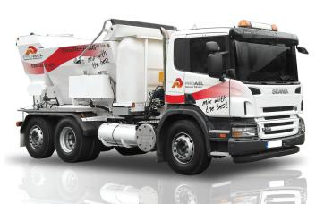
Designed for a shorter wheel-based chassis, the P50 has the smallest footprint of the high-production models. Ideal for tight spaces like urban roadways, but with the same throughput capacity of larger models. The P50 Commander promises a more capable, more precise and more responsive mixing experience - every time.
